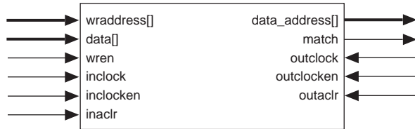
Figure 23. APEX 20KE CAM Block Diagram
