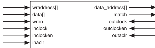
Figure 23. APEX 20KC CAM Block Diagram
