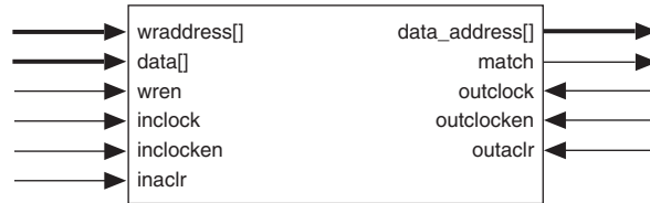
Figure 23. APEX 20KC CAM Block Diagram
