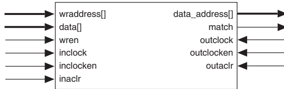
Figure 23. APEX 20KC CAM Block Diagram
