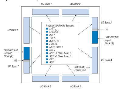
Figure 29. APEX 20KE I/O Banks
