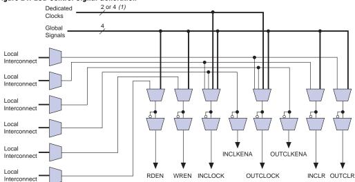
Figure 24. ESB Control Signal Generation
