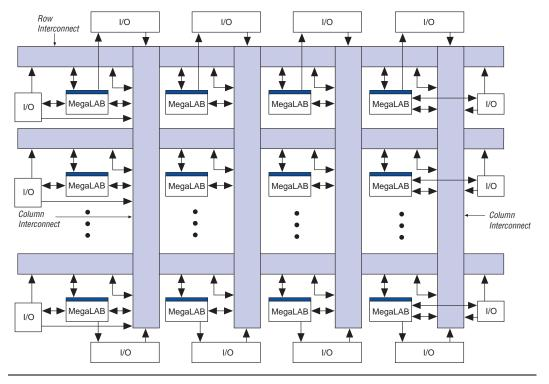
Figure 9. APEX 20K Interconnect Structure
