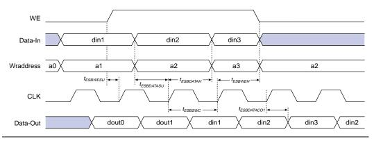
Figure 40 shows the timing model for bidirectional I/O pin timing.
