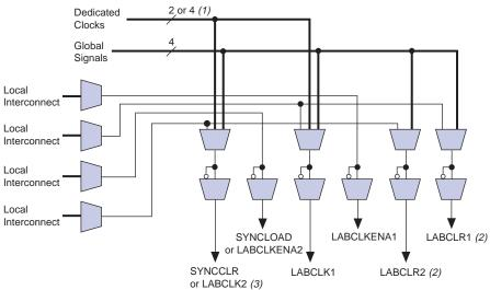
Figure 4. LAB Control Signal Generation
