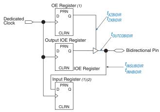
Figure 40. Synchronous Bidirectional Pin External Timing
