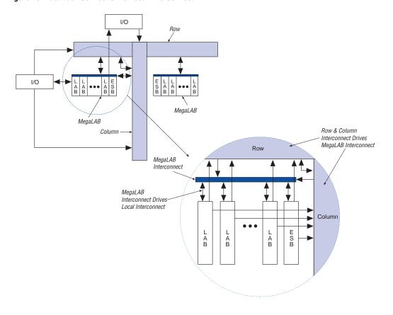
Figure 11 shows the intersection of a row and column interconnect, and how these forms of interconnects and LEs drive each other.
