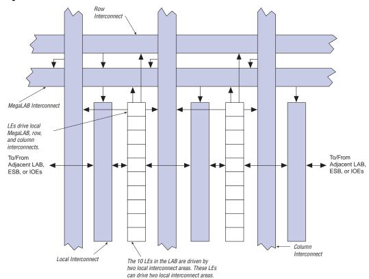
Each LAB contains dedicated logic for driving control signals to its LEs and ESBs. The control signals include clock, clock enable, asynchronous clear, asynchronous preset, asynchronous load, synchronous clear, and synchronous load signals. A maximum of six control signals can be used at a time. Although synchronous load and clear signals are generally used when implementing counters, they can also be used with other functions.
