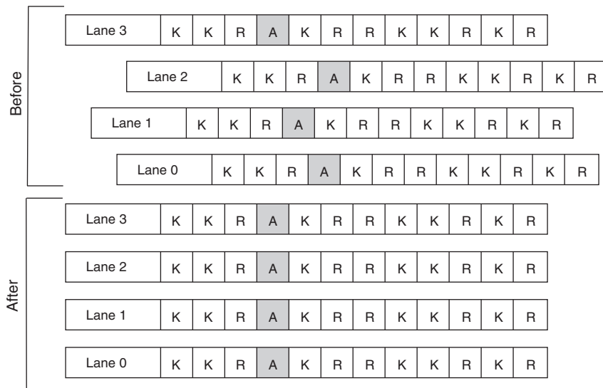
Figure 2–19. Before and After the Channel Aligner
