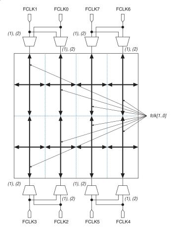
Figure 2–45. EP1S30 Device Fast Regional Clock Pin Connections to Fast Regional Clocks
