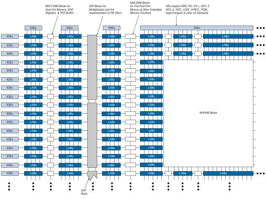
The number of M512 RAM, M4K RAM, and DSP blocks varies by device along with row and column numbers and M-RAM blocks. Table 2–1 lists the resources available in Stratix devices.
