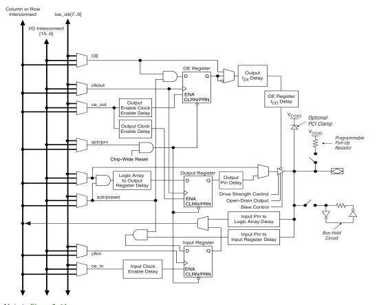
Figure 2–64. Stratix IOE in Bidirectional I/O Configuration Note (1)
