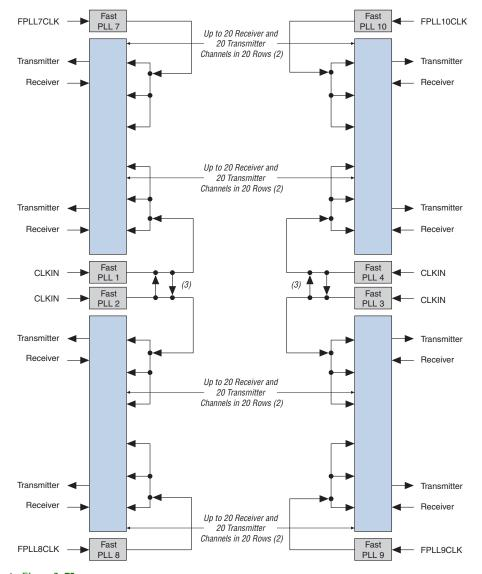
Figure 2-75. Fast PLL & Channel Layout in the EP1S30 to EP1S80 Devices Note (1)
