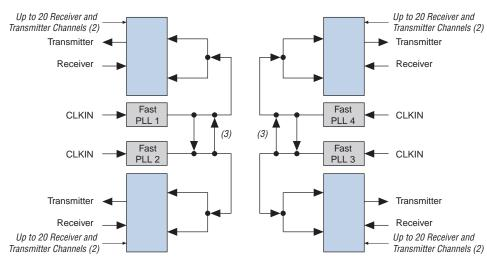
Figure 2–74. Fast PLL & Channel Layout in the EP1\$10, EP1\$20 or EP1\$25 Devices Note (1)
