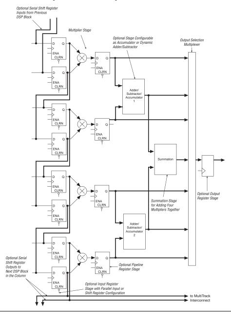
Figure 2-30. DSP Block Diagram for 18 × 18-Bit Configuration
