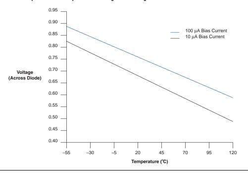
**Temperature Sensing Diode**
