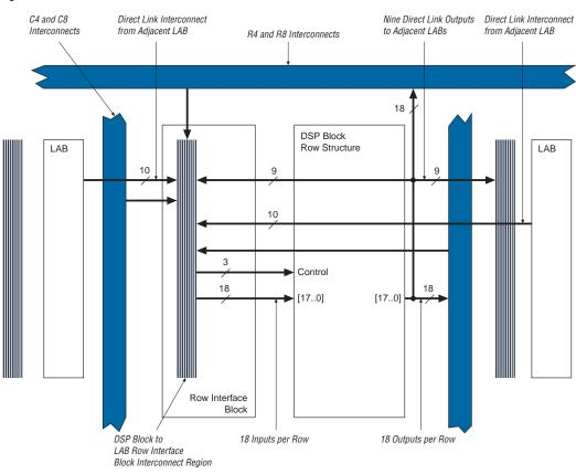
Figure 2-41. DSP Block Interface to Interconnect
