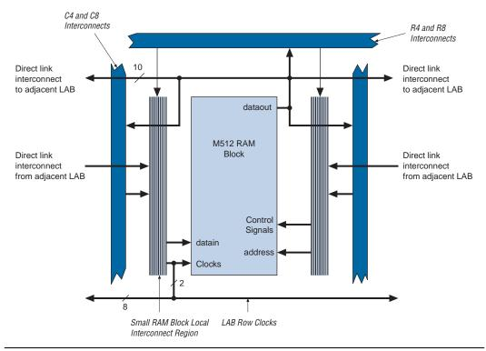
Figure 2-16. M512 RAM Block LAB Row Interface
