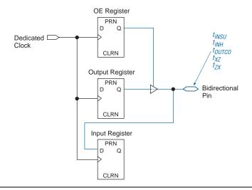
All external timing parameters reported in this section are defined with respect to the dedicated clock pin as the starting point. All external I/O timing parameters shown are for 3.3-V LVTTL I/O standard with the 24-mA current strength and fast slew rate. For external I/O timing using standards other than LVTTL or for different current strengths, use the I/O standard input and output delay adders in Tables 4–103 through 4–108.
