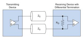
I/O banks on the left and right side of the device support LVDS receiver (far-end) differential termination.
