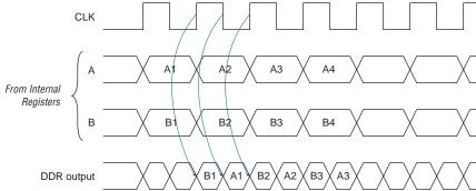
The Stratix IOE operates in bidirectional DDR mode by combining the DDR input and DDR output configurations. Stratix device I/O pins transfer data on a DDR bidirectional bus to support DDR SDRAM. The negative-edge-clocked OE register holds the OE signal inactive until the falling edge of the clock. This is done to meet DDR SDRAM timing requirements.
