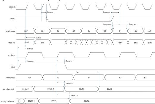
Figure 4–3. Dual-Port RAM Timing Microparameter Waveform
