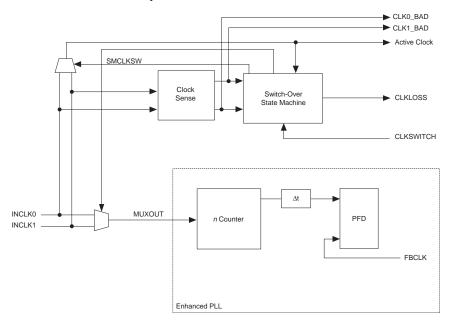
Figure 2-53. Clock Switchover Circuitry
