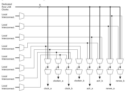
Figure 2-19. M-RAM Block Control Signals
