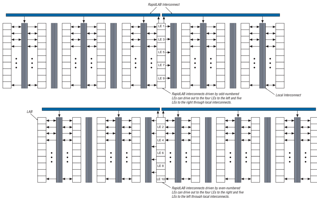
Figure 14. RapidLAB Interconnect Connections
