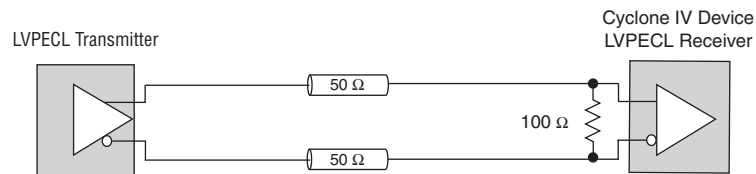
Figure 6-19. LVPECL DC-Coupled Termination (1)
