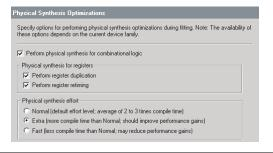
The compiled design shows a performance increase in the FPGA, running at an  $f_{MAX}$  of 74.34 MHz, requiring additional LE resources as a result of the physical synthesis and logic duplication. In this example, you can see how performance can be increased in the Stratix FPGA device at the expense of additional LE resources, as this design's LE resources grew almost 12% over the beginning compilation. The compiled FPGA design's statistics are provided in Table 6–4.
