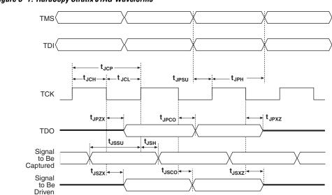
Figure 3-1. HardCopy Stratix JTAG Waveforms
