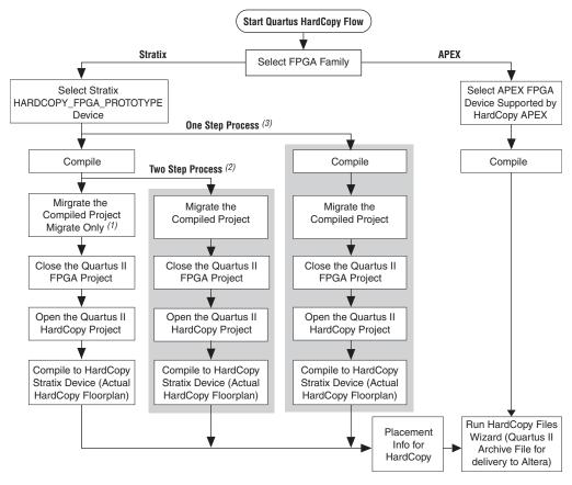
Figure 5-1. HardCopy Stratix and HardCopy APEX Design Flow Diagram
