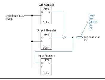
All external timing parameters reported in this section are defined with respect to the dedicated clock pin as the starting point. All external I/O timing parameters shown are for 3.3-V LVTTL I/O standard with the 4-mA current strength and fast slew rate. For external I/O timing using standards other than LVTTL or for different current strengths, use the I/O standard input and output delay adders in the *Stratix Device Handbook*.
