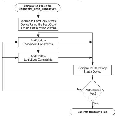
Figure 5-6. Placement Constraints Flow for HardCopy Stratix Devices
