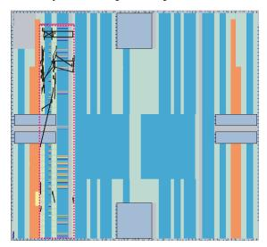
Figure 6–6. Vertically Stretched LogicLock Region
