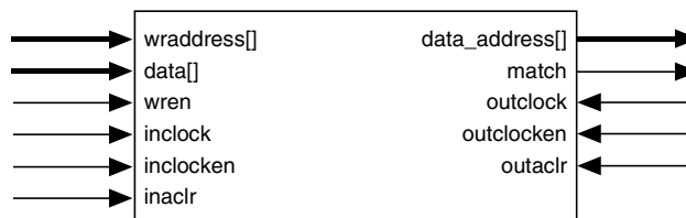
Figure 23. APEX 20KC CAM Block Diagram
