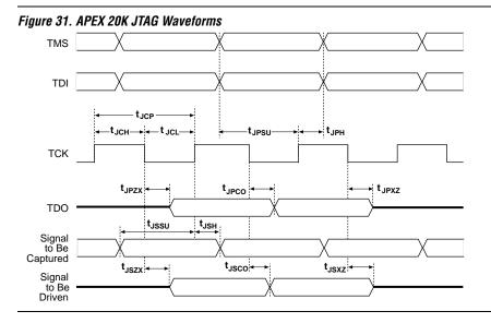
Table 22 shows the JTAG timing parameters and values for APEX 20K devices.
