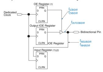
Figure 40. Synchronous Bidirectional Pin External Timing
