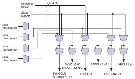
Figure 4. LAB Control Signal Generation
