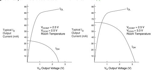
Figure 34. Output Drive Characteristics of APEX 20K Device Note (1)
