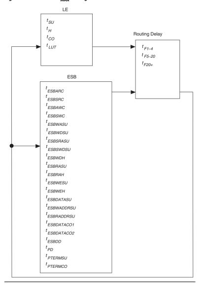
Figure 37. APEX 20KE  $f_{MAX}$  Timing Model
