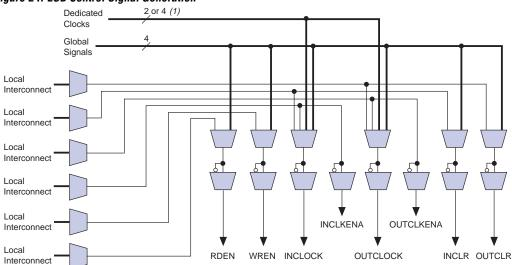
Figure 24. ESB Control Signal Generation
