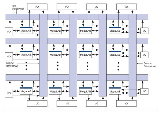
Figure 9. APEX 20K Interconnect Structure
