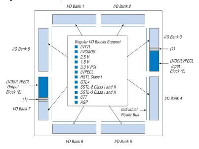
Figure 29. APEX 20KE I/O Banks
