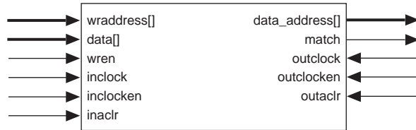
Figure 23. APEX 20KE CAM Block Diagram
