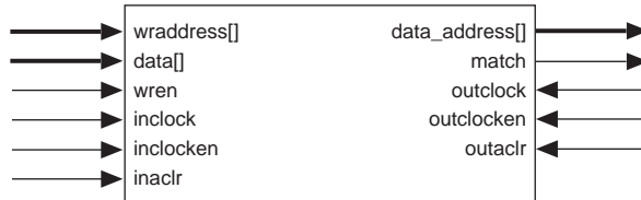
Figure 23. APEX 20KE CAM Block Diagram
